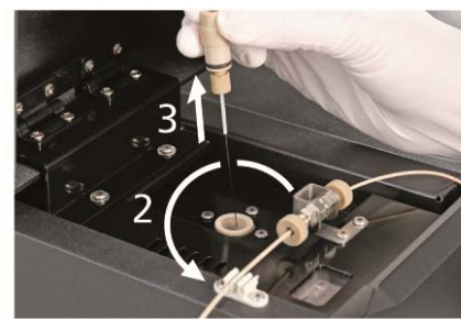
ESI Capillary source replacement
